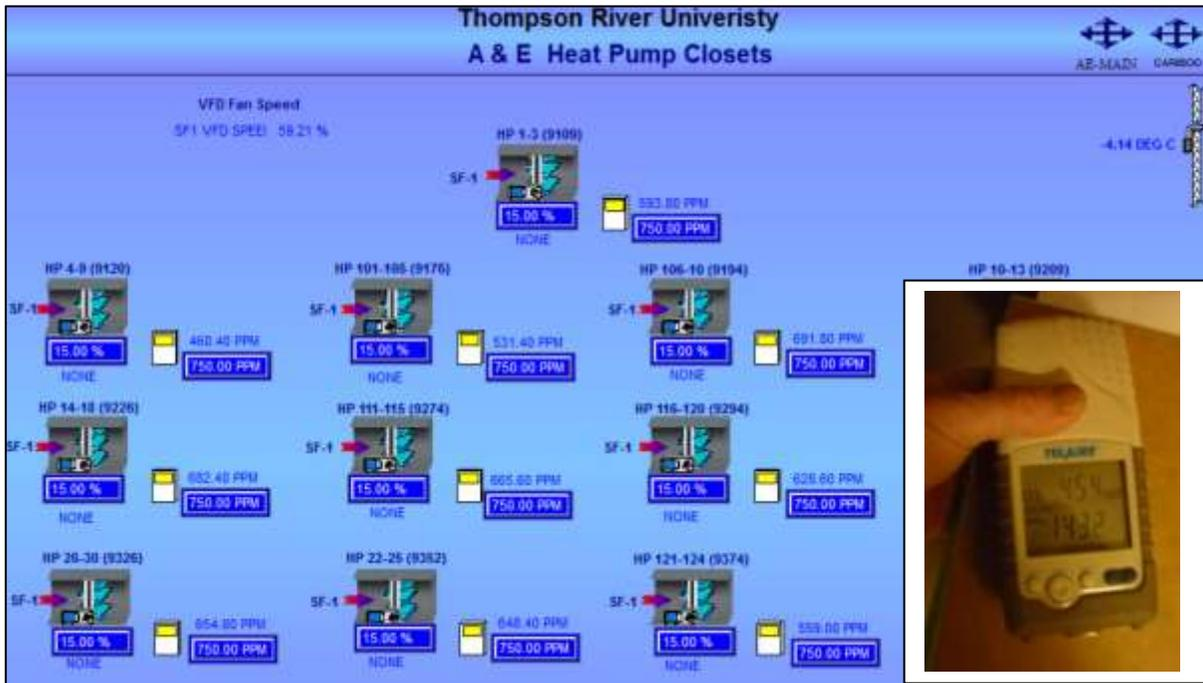
Figure 8: Heat Pump Operational Parameters from DDC & Measured CO2 Concentration
