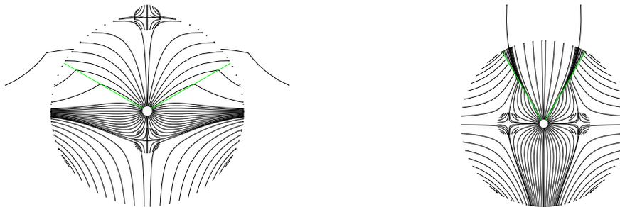
(a) Example of a borderline run with two stagnation points. The parameters include a well suction of 25 inWC, a landfill radius of 25 m, a generation rate or 5000 scfm, permeabilities of  $1e-06 \text{ m}^2$  and  $1e-07 \text{ m}^2$  for the top and bottom sectors respectively, and a boundary angle of  $\pi/6$ .
