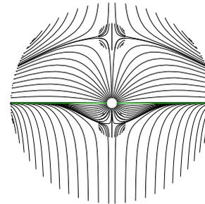
(f) An example of a satisfactory Type II run with two stagnation points and permeabilities of  $1e-08 \text{ m}^2$  and  $1e-09 \text{ m}^2$  for the top and bottom sectors respectively.
