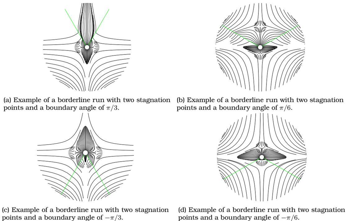
Figure 19: Comparison of borderline runs which include moderate gaps within the figure. The four landfill examples have a suction level of 5 inWC, a landfill diameter of 25 m, and a generation rate of 50 scfm. The permeabilities of Subfigures 19a and 19b are  $1e - 08 m^2$  and  $1e - 09 m^2$  for the top and bottom sectors respectively. The permeabilities of Subfigures 19c and 19d are  $1e - 09 m^2$  and  $1e - 10 m^2$  for the top and bottom sectors respectively.
