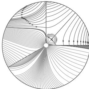
(c) Example of a satisfactory run with one stagnation point and boundary angles at  $\pi/2$ ,  $7\pi/6$  and  $2\pi$ . Landfill parameters include a suction level of 25 inWC, a landfill diameter of 5 m, a generation rate of 500 scfm and permeabilities of  $1e-06 \text{ m}^2$ ,  $1e-08 \text{ m}^2$  and  $1e-07 \text{ m}^2$ .
