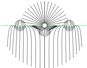
(c) An example of a Type I borderline run with three stagnation points. This example has a suction level of 25 inWC, a landfill radius of 50 m, a generation rate of 500 scfm, and permeabilities of  $1e-08 \text{ m}^2$  and  $1e-09 \text{ m}^2$  for the top and bottom sectors respectively.
