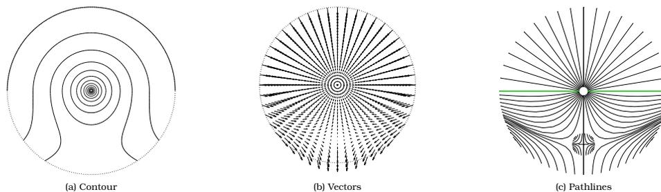
Figure 3: Three visualization methods used to visualize fluid flow through a porous medium.
