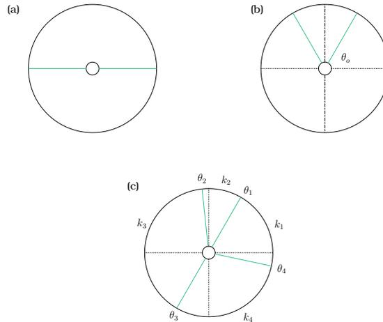
Figure 2: Sector configurations and counting notation of landfill well cross-sections for (a) semicircular sectors, (b) two unequal sectors and (c) arbitrary number of sectors (Nec and Huculak, 2020).
