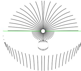
(b) An example of an unsatisfactory Type II run with one stagnation point. This example has a suction level of 25 inWC, a landfill radius of 50 m, a generation rate of 50 scfm, and permeabilities of  $1e-08 \text{ m}^2$  and  $1e-09 \text{ m}^2$  for the top and bottom sectors respectively.
