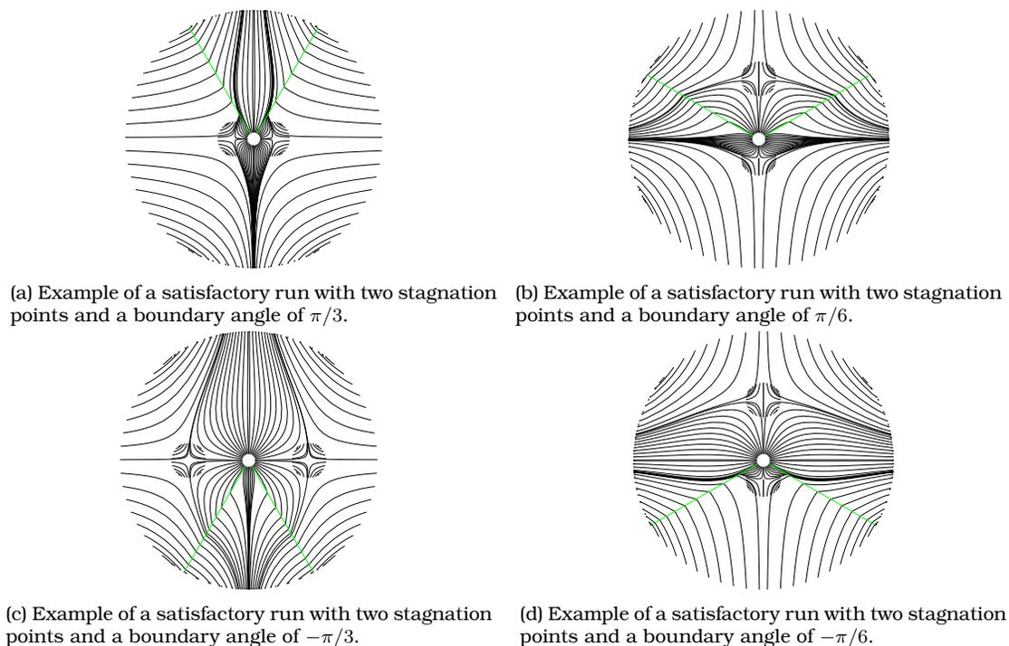
Figure 17: Comparison of satisfactory runs with two stagnation points. The four landfill examples have a suction level of 5 inWC, a landfill diameter of 25 m, a generation rate of 500 scfm and permeabilities of  $1e-07 \text{ m}^2$  and  $1e-08 \text{ m}^2$  for the top and bottom sectors respectively.
