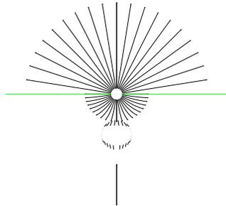
(a) An example of an unsatisfactory Type I run with one stagnation point. This example has a suction level of 25 inWC, a landfill radius of 50 m, a generation rate of 50 scfm, and permeabilities of  $1e-08 \text{ m}^2$  and  $1e-09 \text{ m}^2$  for the top and bottom sectors respectively.
