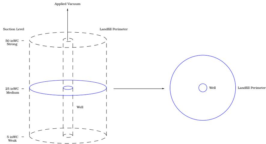
Figure 1: Simplified three dimensional and cross section examples of a generic landfill set-up. Note: In a physical landfill wells can be horizontal, vertical or a combination network. The dimensions in this figure are not to scale and realistic suction variation is non-linear.
