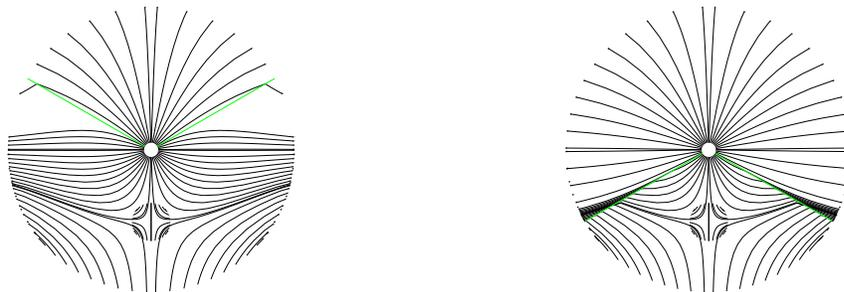
(a) Example of a satisfactory run with one stagnation point and a boundary angle of  $\pi/6$ . (b) Example of a satisfactory run with one stagnation point and a boundary angle of  $-\pi/6$ .
