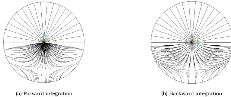
Figure 5: Examples of forward and backward integration of pathlines for a landfill with two equal sectors, generated in VU.
