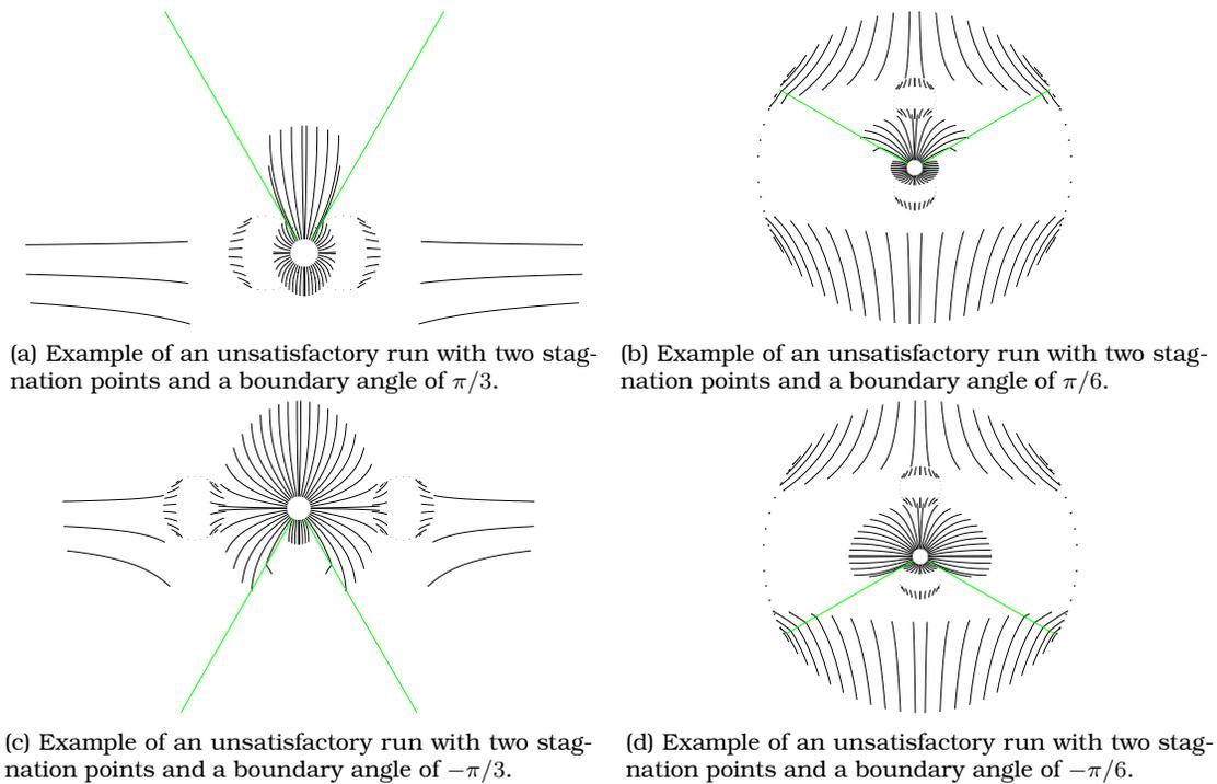
Figure 21: Comparison of unsatisfactory runs with major gaps in the pathline integration. The four landfill examples have a suction level of 5 inWC, a landfill diameter of 50 m, a generation rate of 50 scfm and permeabilities of  $1e-08 \text{ m}^2$  and  $1e-09 \text{ m}^2$  for the top and bottom sectors respectively.
