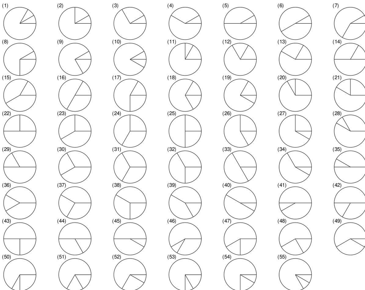
Figure 23: All possible geometries for a landfill with three sectors given the angles available (Figure 22).
