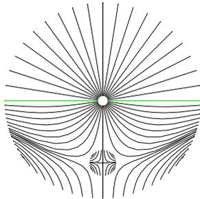
(c) An example of a satisfactory Type I run with one stagnation point and permeabilities of  $1e-07 \text{ m}^2$  and  $1e-08 \text{ m}^2$  for the top and bottom sectors respectively.
