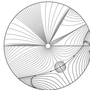
(b) Example of a satisfactory run with one stagnation point and boundary angles at  $2\pi/6$ ,  $\pi$  and  $2\pi$ . Landfill parameters include a suction level of 5 inWC, a landfill diameter of 5 m, a generation rate of 500 scfm and permeabilities of  $1e-07 \text{ m}^2$ ,  $1e-08 \text{ m}^2$  and  $1e-06 \text{ m}^2$ .
