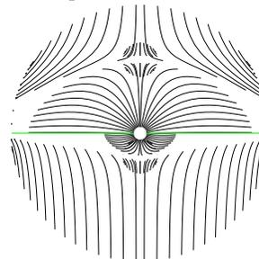
(d) An example of a Type II borderline run with two stagnation points. This example has a suction level of 5 inWC, a landfill radius of 25 m, a generation rate of 50 scfm, and permeabilities of  $1e-08 \text{ m}^2$  and  $1e-09 \text{ m}^2$  for the top and bottom sectors respectively.
