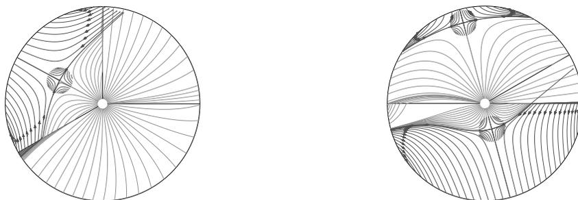
(a) Example of a borderline run with one stagnation point and boundary angles at  $\pi/2$ ,  $7\pi/6$  and  $2\pi$ . Landfill parameters include a suction level of 5 inWC, a landfill diameter of 5 m, a generation rate of 500 scfm and permeabilities of  $1e-06 \text{ m}^2$ ,  $1e-05 \text{ m}^2$  and  $1e-07 \text{ m}^2$ .
