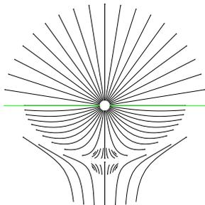
(a) An example of a Type I borderline run with one stagnation point. This example has a suction level of 5 inWC, a landfill radius of 25 m, a generation rate of 50 scfm, and permeabilities of  $1e-07 \text{ m}^2$  and  $1e-08 \text{ m}^2$  for the top and bottom sectors respectively.
