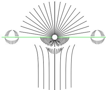
(c) An example of an unsatisfactory Type I run with three stagnation points. This example has a suction level of 5 inWC, a landfill radius of 25 m, a generation rate of 50 scfm, and permeabilities of  $1e-08 \text{ m}^2$  and  $1e-09 \text{ m}^2$  for the top and bottom sectors respectively.
