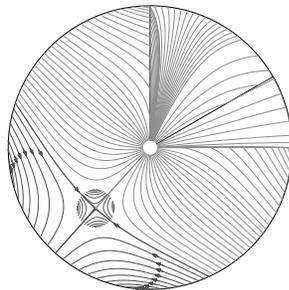
(a) Example of a satisfactory run with one stagnation point and boundary angles at  $\pi/6$ ,  $\pi/3$  and  $2\pi$ . Landfill parameters include a suction level of 25 inWC, a landfill diameter of 5 m, a generation rate of 50 scfm and permeabilities of  $1e-06 \text{ m}^2$ ,  $1e-07 \text{ m}^2$  and  $1e-08 \text{ m}^2$ .
