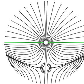
(d) An example of a satisfactory Type II run with one stagnation point and permeabilities of  $1e-07 \text{ m}^2$  and  $1e-08 \text{ m}^2$  for the top and bottom sectors respectively.
