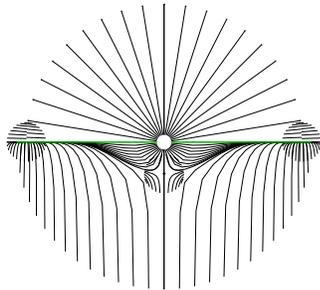
(e) An example of a satisfactory Type I run with three stagnation points and permeabilities of  $1e-08 \text{ m}^2$  and  $1e-09 \text{ m}^2$  for the top and bottom sectors respectively.
