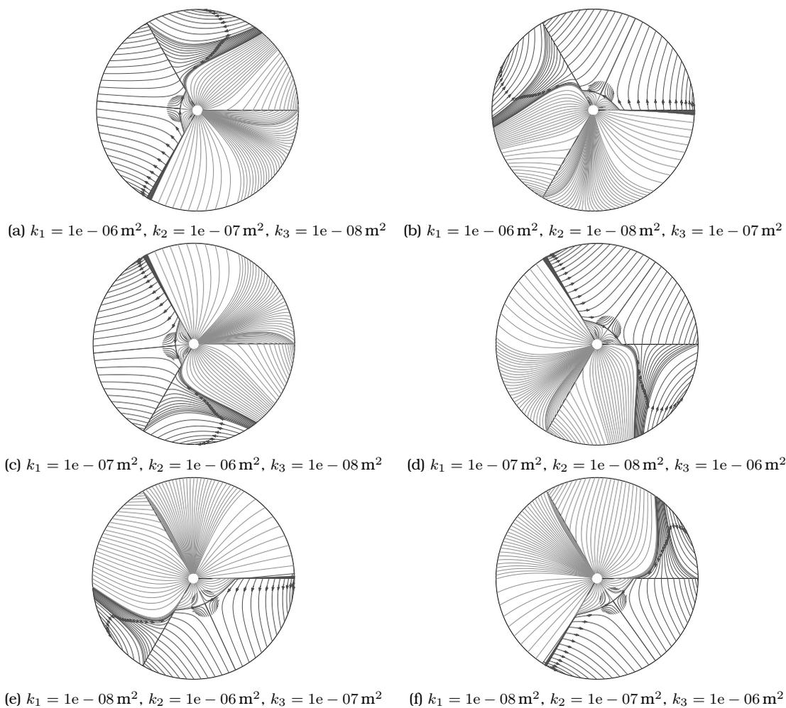
Figure 30: Comparison of how rotation of permeabilities affect the number and location of stagnation points. Landfill parameters include a suction level of 50 inWC, a landfill diameter of 5 m, a generation rate of 5000 scfm, permeabilities of  $1e - 06 \text{ m}^2$ ,  $1e - 07 \text{ m}^2$  and  $1e - 08 \text{ m}^2$  and boundary angles of  $2\pi/3$ ,  $4\pi/3$ , and  $2\pi$ .
