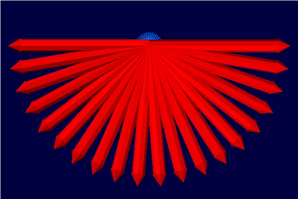
Figure 4: Vector representation created using VU, showing the issues occurring when the magnitude of the vectors is depicted to scale. Here the large red arrows represent gas flow with a high velocity immediately around the well, which completely obstructs the small blue arrows representing the gas flow with lower velocity around the perimeter of the landfill.
