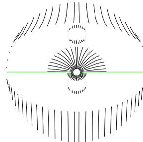
(d) An example of an unsatisfactory Type II run with two stagnation points. This example has a suction level of 5 inWC, a landfill radius of 50 m, a generation rate of 50 scfm, and permeabilities of  $1e-08 \text{ m}^2$  and  $1e-09 \text{ m}^2$  for the top and bottom sectors respectively.
