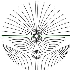
(b) An example of a Type II borderline run with one stagnation point. This example has a suction level of 5 inWC, a landfill radius of 25 m, a generation rate of 50 scfm, and permeabilities of  $1e-07 \text{ m}^2$  and  $1e-08 \text{ m}^2$  for the top and bottom sectors respectively.
