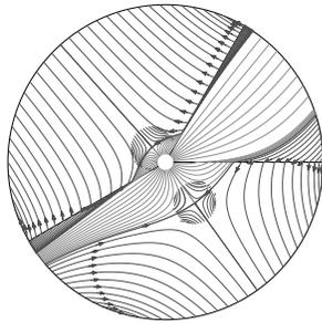
(c) Example of a satisfactory run with two stagnation points and boundary angles at  $\pi/3$ ,  $7\pi/6$  and  $2\pi$ . Landfill parameters include a suction level of 25 inWC, a landfill diameter of 25 m, a generation rate of 500 scfm and permeabilities of  $1e-08 \text{ m}^2$ ,  $1e-07 \text{ m}^2$  and  $1e-09 \text{ m}^2$ .
