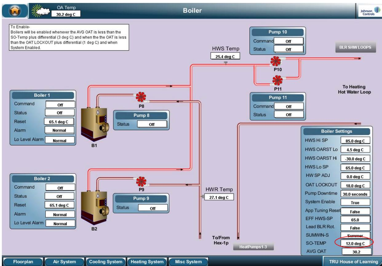
Figure: Switchover temp is 12°C in the cooling season and is reset manually by the operator
