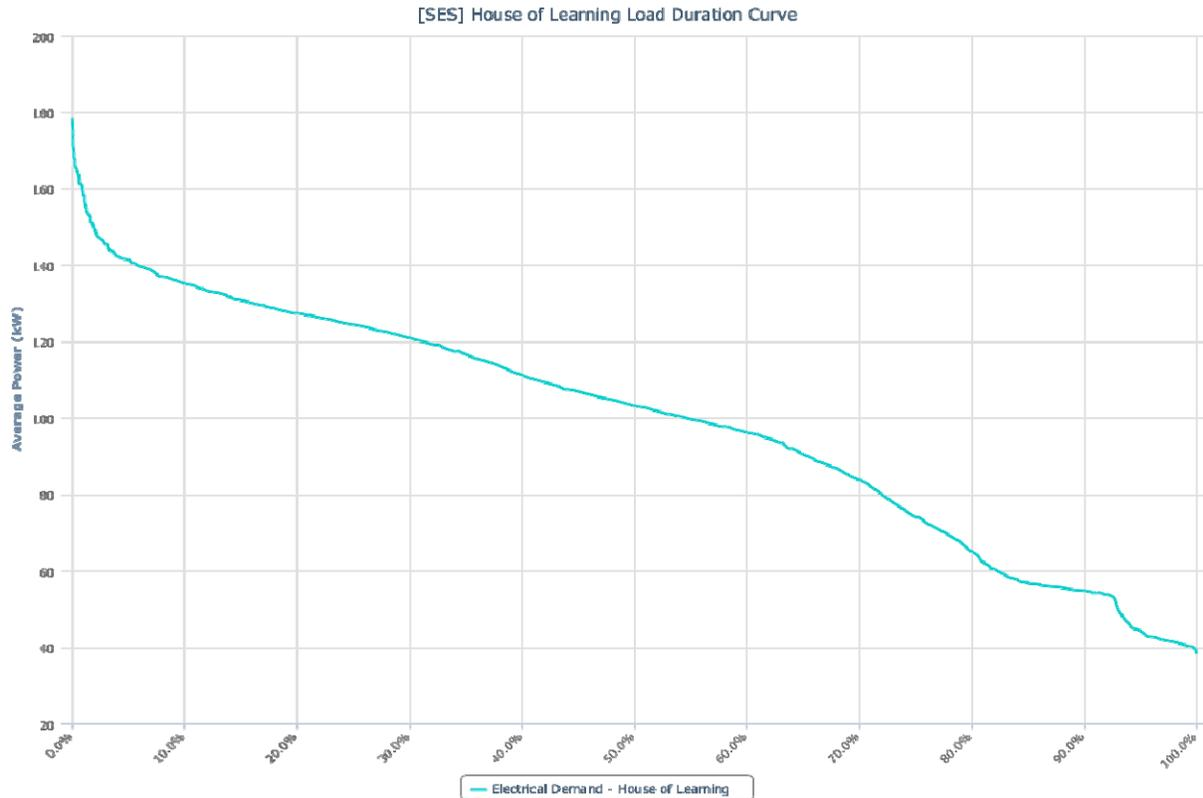
**Figure: Pulse trend indicates demand may be limited to approximately 150 kW**
