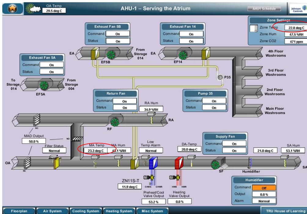
Figure: DDC screenshot of AHU1 heat recovery system
