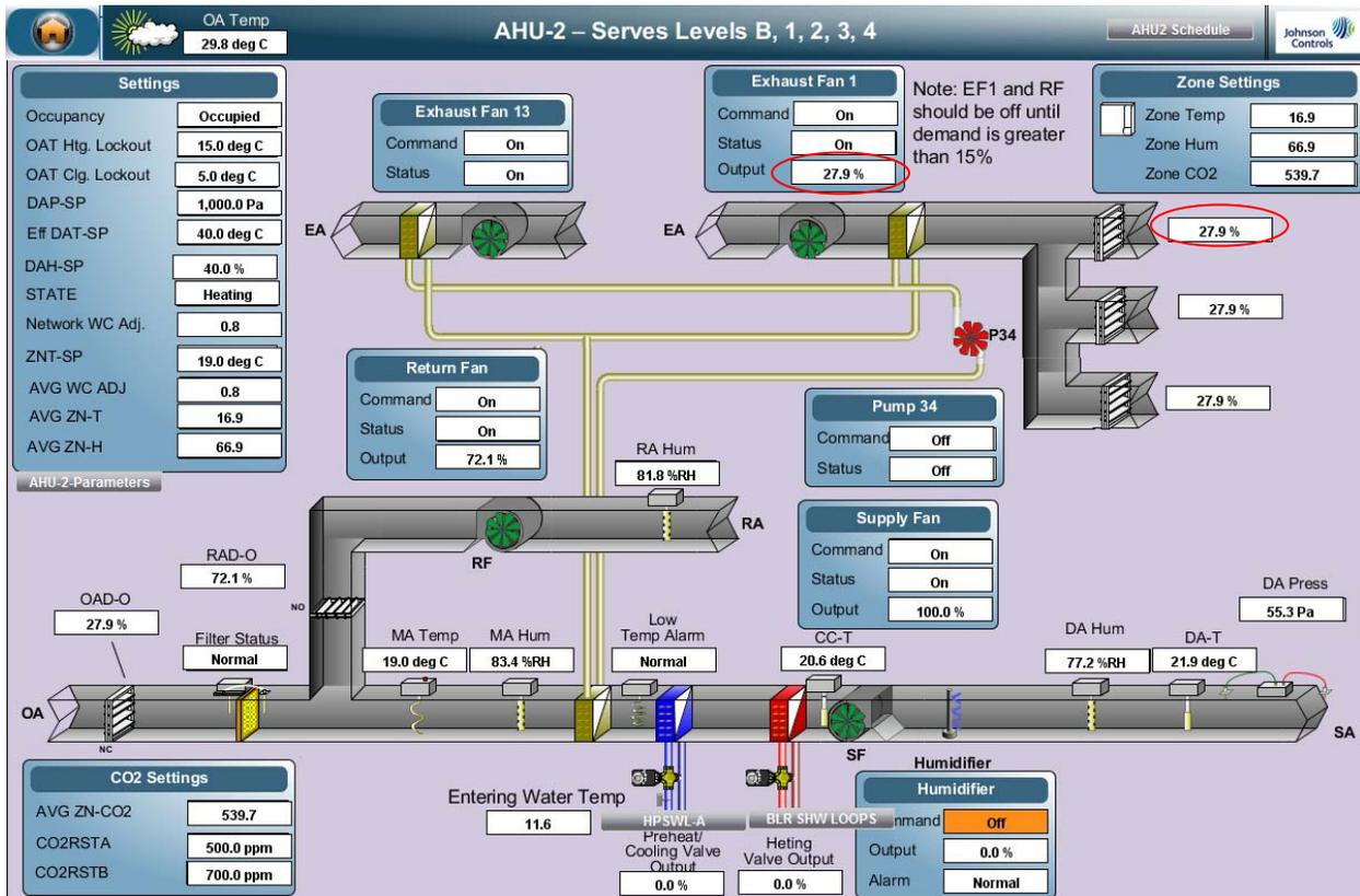
Figure: Relief fan damper position controlled to fan speed
