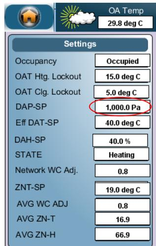
**Figure: High duct air pressure setpoint for AHU 2**
