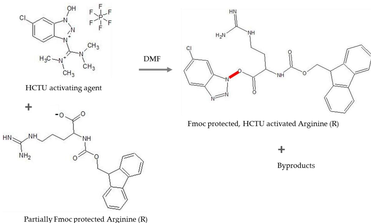
**Reaction 2: Fmoc protected arginine amino acid that has been treated with the organic base NMM undergoing activation by the coupling agent HCTU.**
