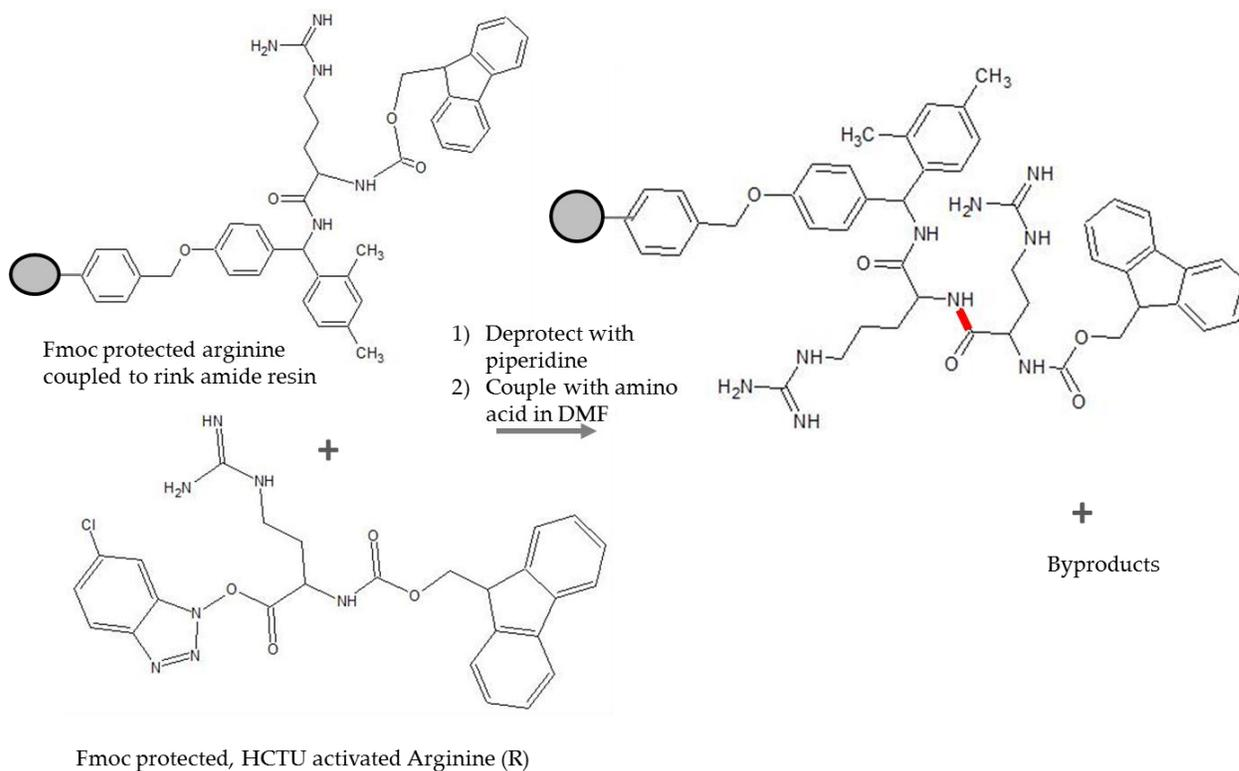
**Reaction 4: Arginine amino acid coupling with Fmoc protected and HCTU activated Arginine. The result is two arginine residues in sequence attached to the rink amide resin. The second arginine of the sequence is still Fmoc protected.**
