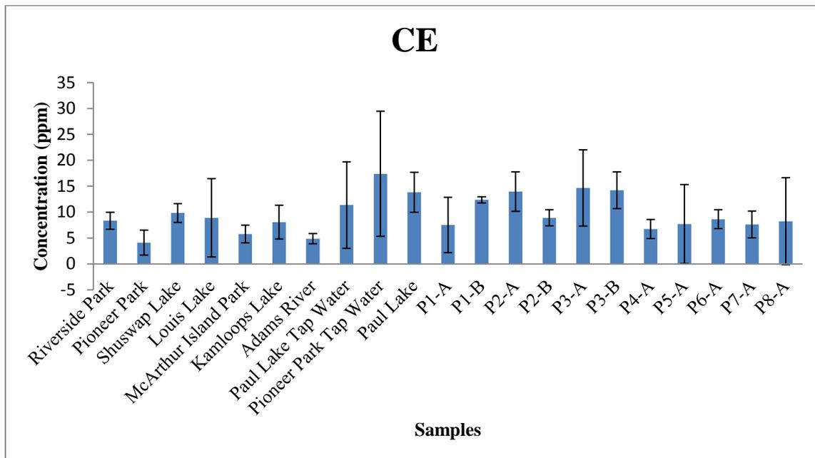
Figure E.1. Concentration of BPA in samples analyzed by CE
