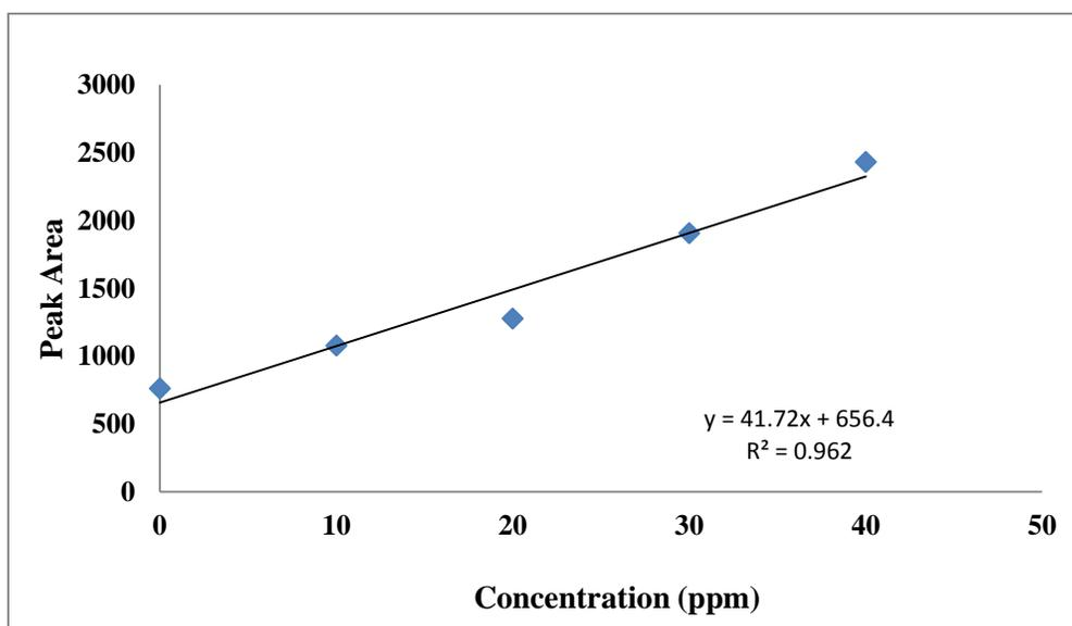
Figure 5.1. BPA standard addition plot by CE
