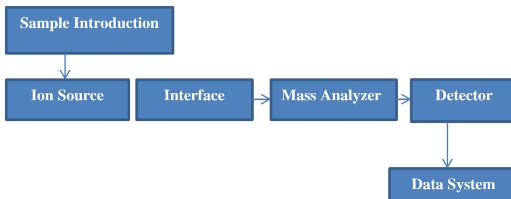
Figure 2.6. Schematic of mass spectrometer
