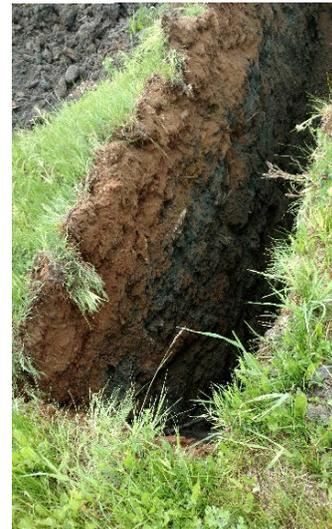
Figure 2.3 Pictures showing a) sampling of the topsoil stockpile in QR mill via mechanical digger and b) a sample hole exposing part of the topsoil profile
