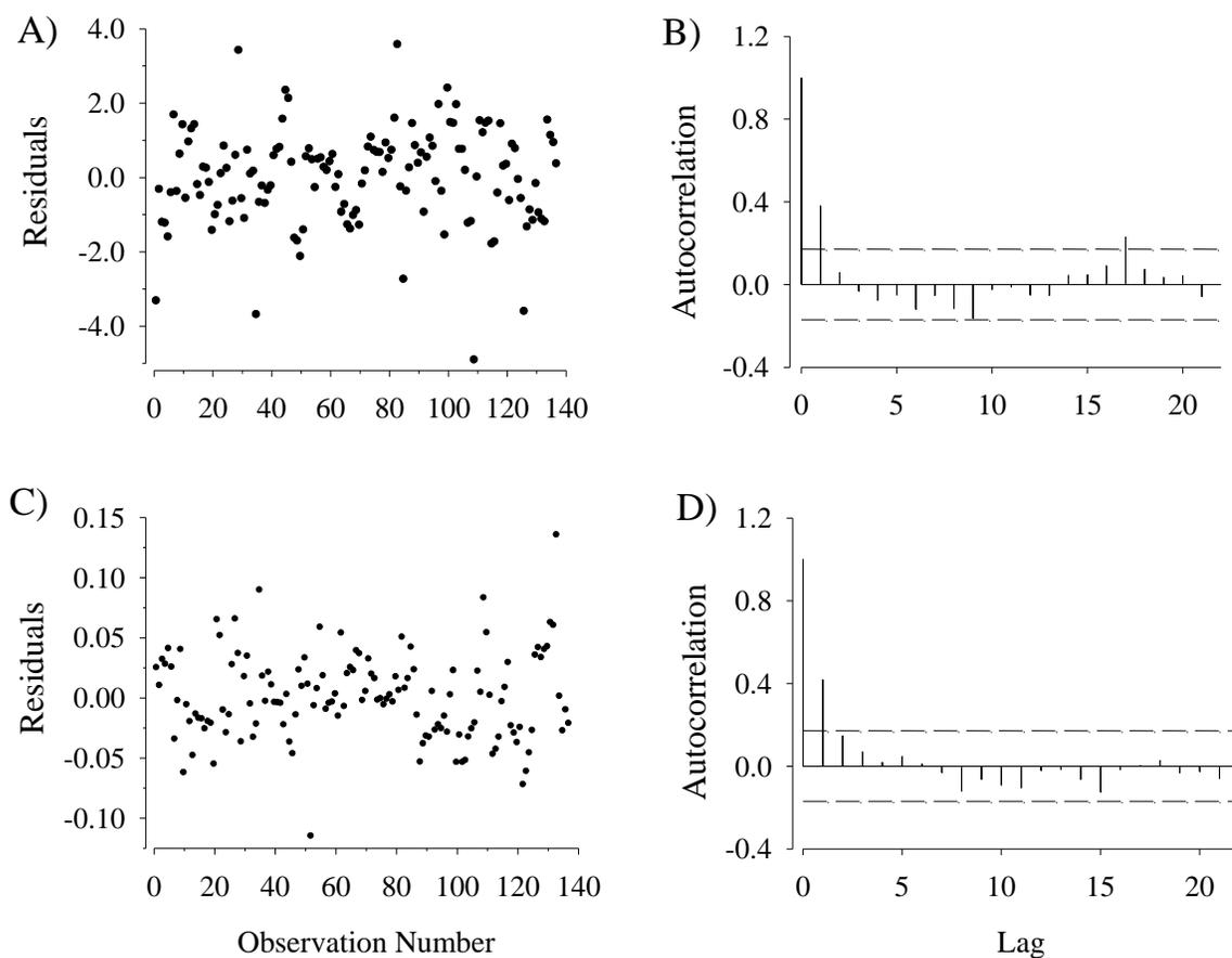
**Figure A.1.** Results of autocorrelation analysis of residuals from multiple regression models predicting intertidal temperature (A&B) and intertidal relative humidity (C&D). A&C represent scatterplots of the model residuals as a function of time in the form of consecutive observations. B&D represent bar plots of autocorrelation of residuals as a function of lag time. Bars outside the limits of the 95% CI (dashed lines in B&D) suggest significant autocorrelation at the associated lag value.
