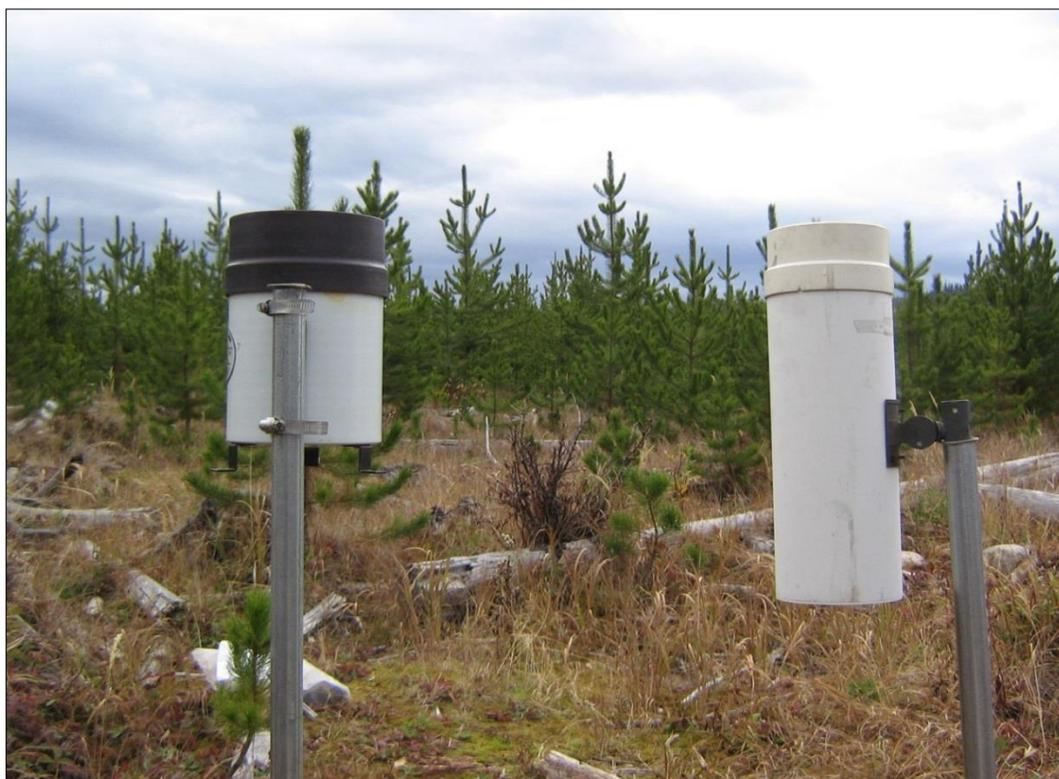
**Figure 3.4:** The Onset<sup>®</sup> tipping bucket rain gauge (left) and Meteorological Service of Canada Type-B rain gauge (right) used in this study
