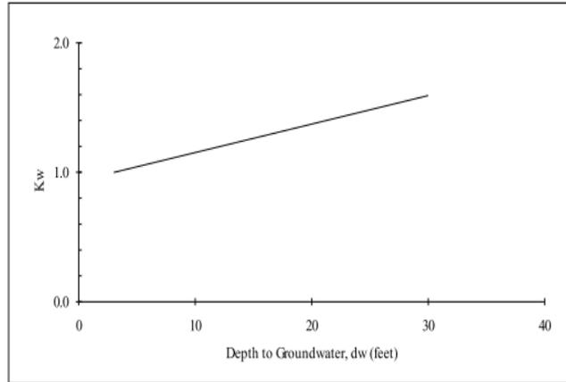
Figure 2-4. Ground water depth correction factor, KW (FEMA 2015).
