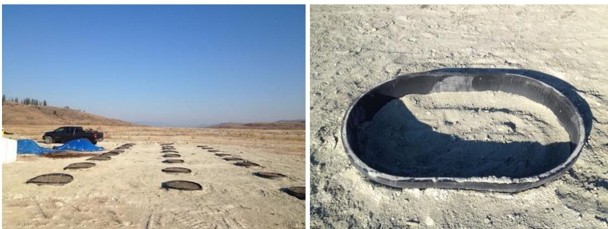
**Figure 3.2.** View of Historic Afton Tailings Storage Facility research plots (left) and individual plot containing unamended tailings (right).
