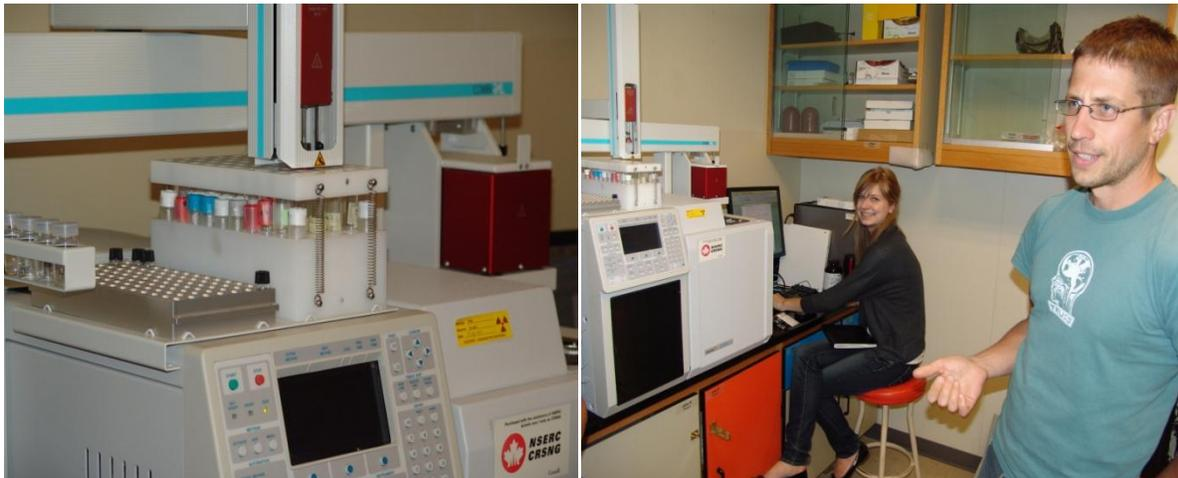
**Figure 2.6.** Measuring methane samples using gas chromatography.
