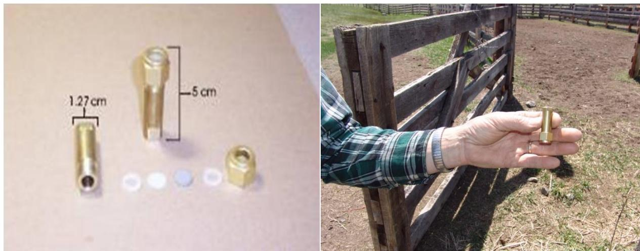
**Figure 2.1.** Permeation tube and components.
