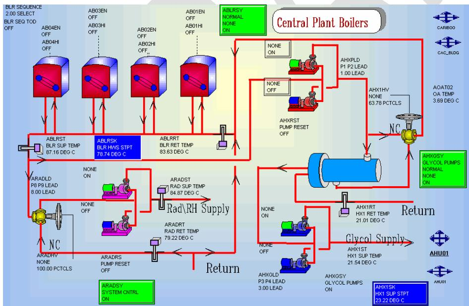
Figure 7: Heating Plant DDC Graphic
