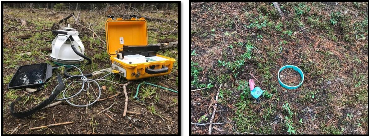
**Figure 3.3:** LI-COR, LI-8100A automated CO<sub>2</sub> soil gas flux system with a direct survey chamber ranged between 0ppm to 20,000ppm and an operating temperature range between -20°C to 45°C. A green soil Collar with a 10 cm inside and 11.4 cm outside diameter, and with 10 cm of length inserted permanently in the soil, and a minimum of 2 cm extension above the soil surface (Li-COR Biosciences 2010a).
