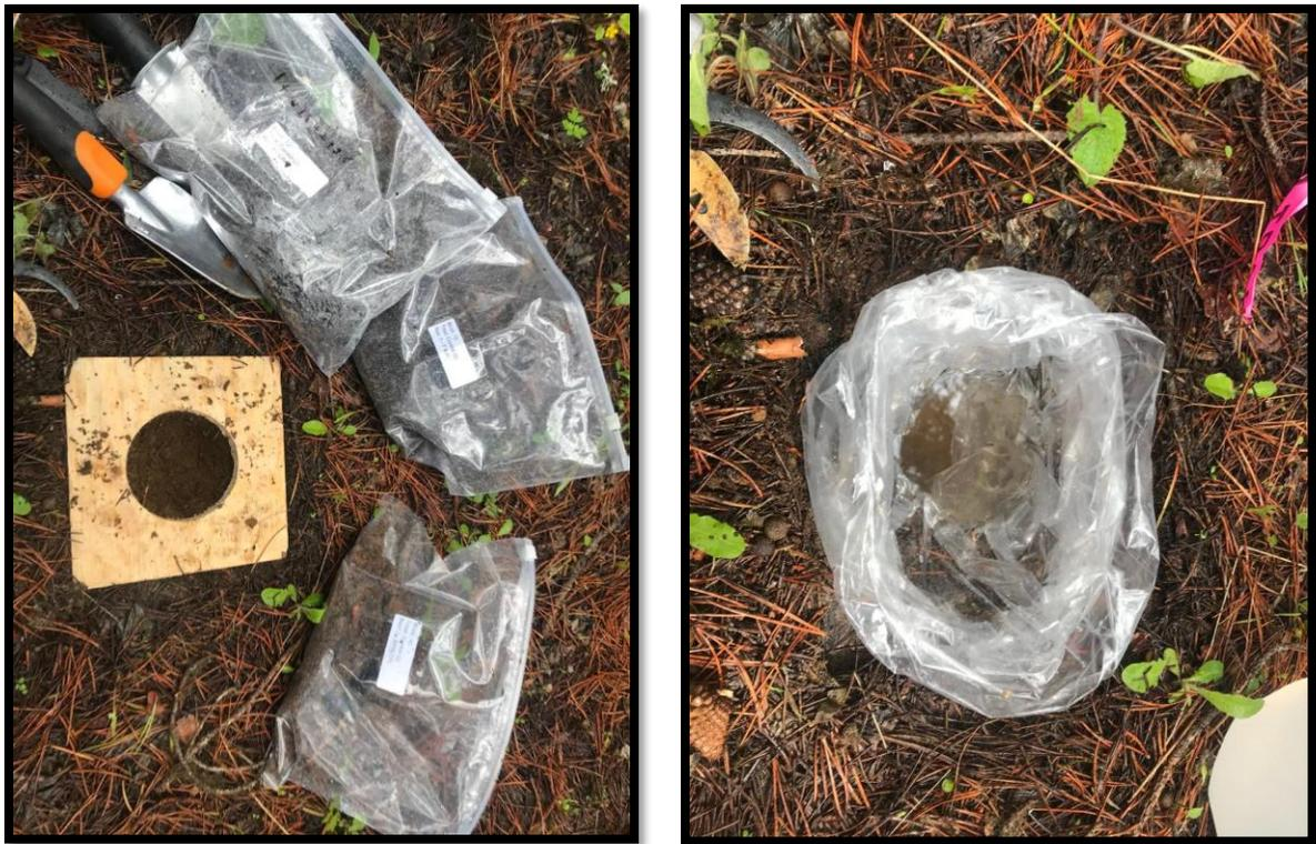
A.12. Excavation method and materials for soil bulk density analysis used post-harvest 2020.
